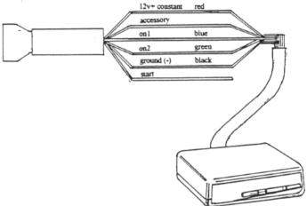
Example 2: Some cars require 1 wire to be energized when the key is in the "ON" position. The other wire will go to a wire normally energized in the "ACC" position.
